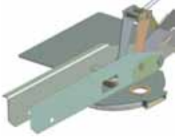
Midsurfacing operations on a thin structure
